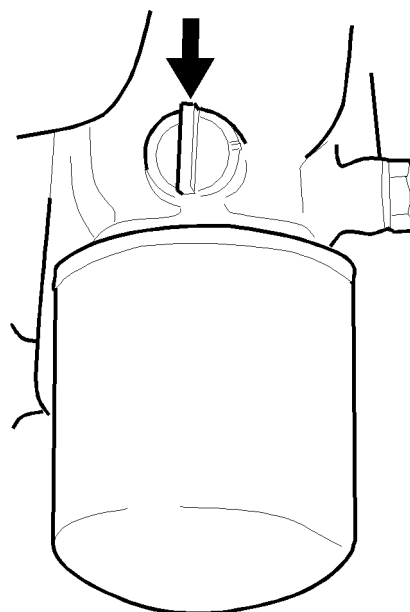
Coolant filter with open valve.
